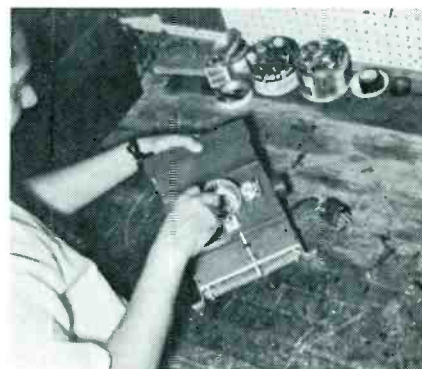
Keeping the cavities clean helps maintain cavity noise at a minimum level.
